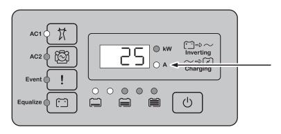
**NOTE:** Unless the inverter/charger settings have been changed, the inverter will charge as if it has a large (> 440 Ah) flooded battery bank (factory default setting). In newly installed systems, adjust the battery charging set points to match the batteries as installed.
