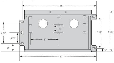
**Note:** If the wall does not have 16-inch on-center studs, you will need to provide adequate support for the Mounting Plates. For example, a sheet of fire-rated plywood can be attached to the wall, and the Mounting Plates can then be attached to plywood.
