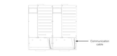
**NOTE:** In a dual-inverter system, install an AC Sync Cable from INV1 to INV2. In a tripleinverter system, daisy-chain an AC Sync Cable from INV1 to INV2 and from INV2 to INV3.
