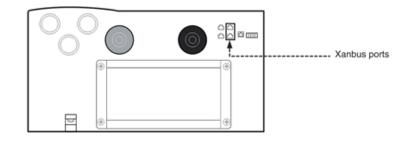
For more information about installing a Xanbus-enabled device as part of a network system, see "The Xanbus Network" on page 119.
