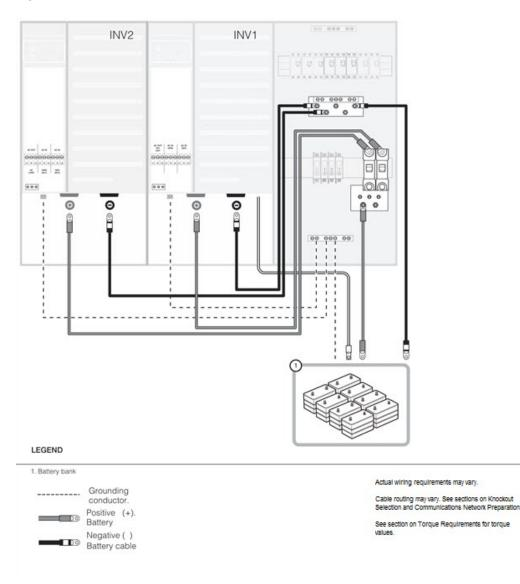
Figure 47 DC Connections to Dual Inverter
