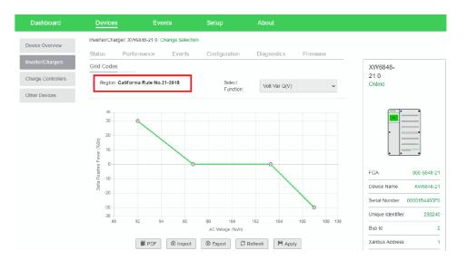
4. Configure the inverter to use an appropriate region code before putting the unit into operating mode.
