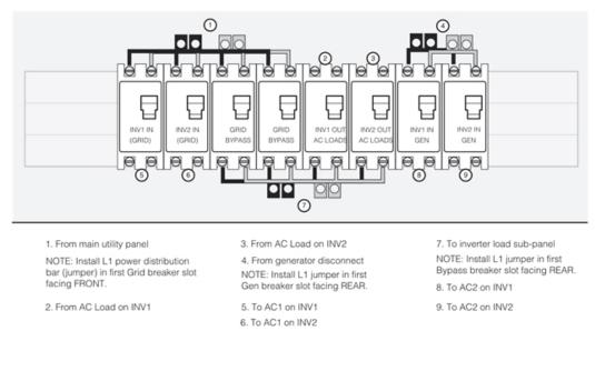
Figure 48 Dual Inverter AC Breaker Arrangement with Multiple AC Input Sources
