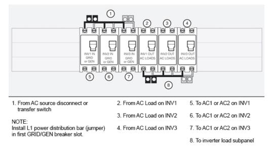
Figure 53 Triple-Inverter AC Breaker Arrangement with Two AC Input Sources
